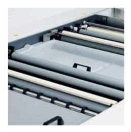
Rollers and brushes are mounted with snap lock bearings, so they can be instantly replaced without tools or the need to re-calibrate pressure.
